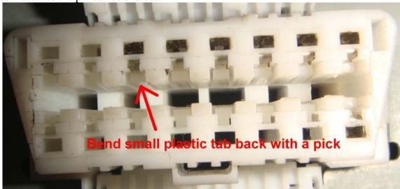
Remove the pin from position 3 and relocate it to position 14.
