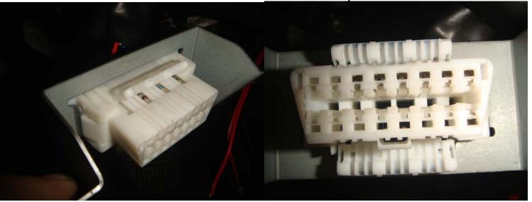
Use a pick or other pointed tool to bend back the retaining clip in the center of the connector so the pin can be slid out.
